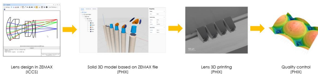
Figure 4 Flowchart of 3D lens fabrication
